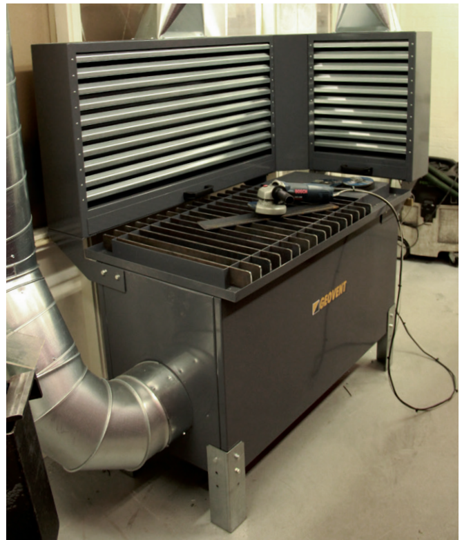
Above, standard table. Lamels are easy to move or changed if needed. Rubber mat can be order.
